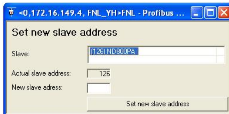
Figure 13: Set Profibus Slave Address
