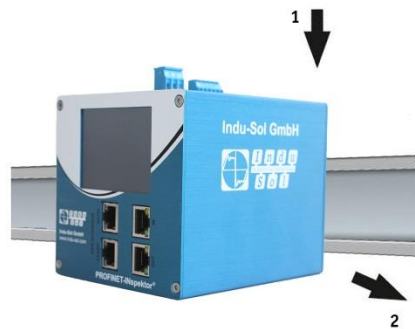
Figure 2: Device installation on top-hat rail
