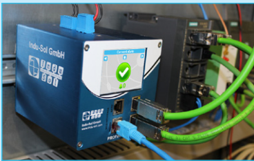
Fig. 1: Installation of the PROFINET-INspektor® NT
