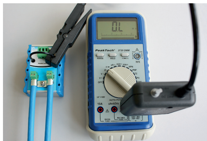
Connection direct current measuring device with multimeter
