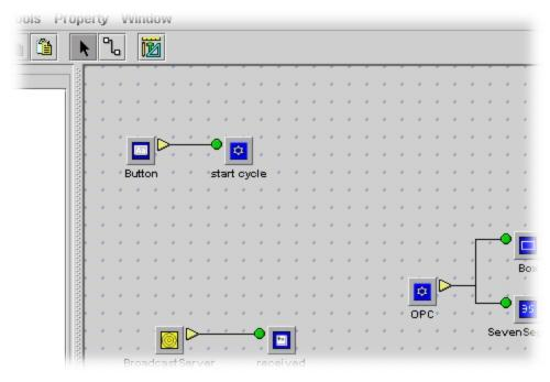
Test this OPC connection by pressing the Cycle Button on the VIBLaces screen. You will need to put VIBLaces into "Run" mode (press the running person button) before you can press the button. When you press the button you should see the Seven Segment display and Box update with the ram position as the Think & Do screen also updates.
