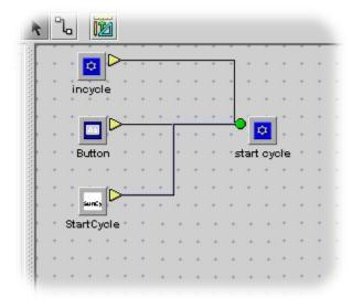
The figure to the left has another OPC bean added to it to read the "InCycle" status of the ram. When the ram is moving the "InCycle" item is high (Boolean true) and then it goes low (Boolean false) when the ram is finished. This is what we need to reset the start cycle signal from the Host to the Think & Do start cycle simulator.
