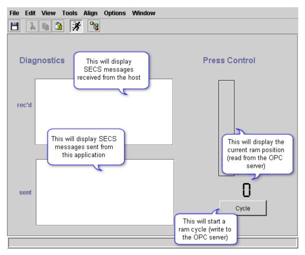
To build this screen, start VIBLaces. You will see a blank Design Window. Add two SwingTextArea beans as shown to display the SECS messages. This will form the basic "diagnostics" of the user interface, so you can see the SECS messages being received and sent. Add the three SwingLabels; change their labels to Diagnostics, rec'd and sent. Add one more SwingLabel for the "Press Control" heading.
