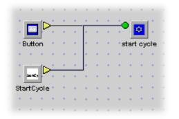
We want to trigger the ram cycle when the StartCycle SECS message is sent to the VIB application. All we need to do is add the S2F42 (StartCycle) message to the logic. Position it near the Cycle Button as shown and quick connect it to the OPC bean that starts the ram cycle. You can test this configuration by going to TransSECS and selecting the S2F41 message and sending it (press the Send Message button). Make sure TransSECS is in Run Mode or you won't have the Send Message button present.
