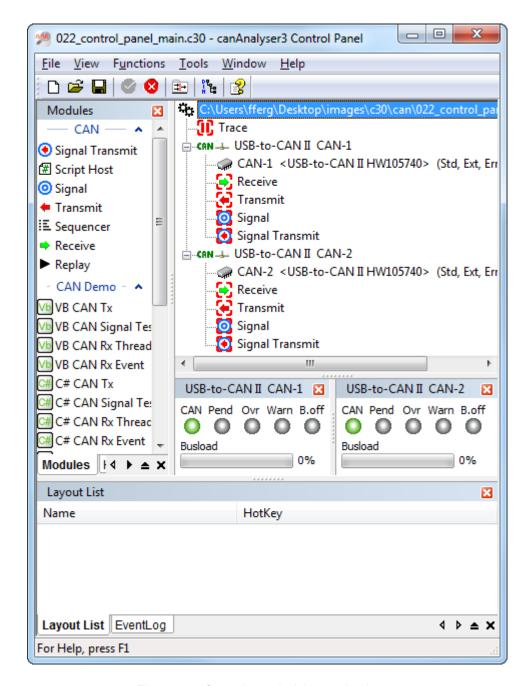
Figure 1.1: Control panel of the canAnalyser
