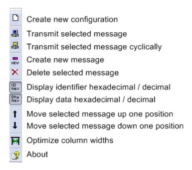
Figure 5.38: Toolbar of the Transmit module
