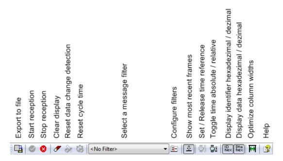
Figure 5.30: Toolbar of the Receive module
