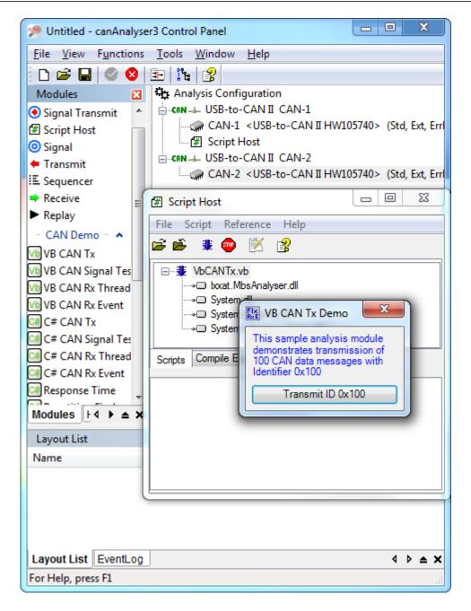
Figure 5.65: GUI and console programming sample executed as script
