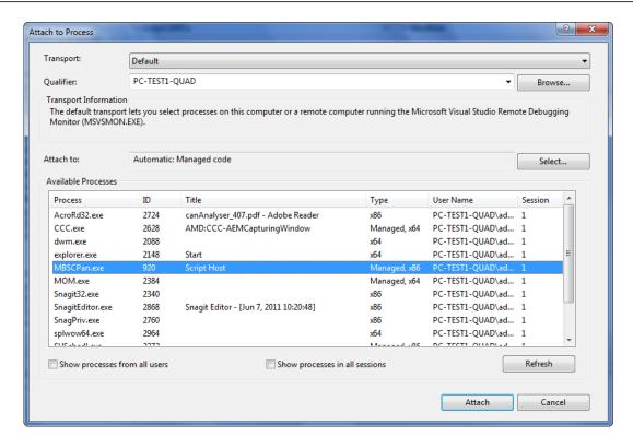
Figure 5.70: Attaching debugger to the canAnalyser
