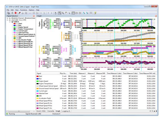
Figure 5.54: Signal module showing Graph View
