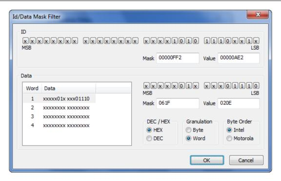
Figure 5.63: Id/Data Mask Filter configuration
