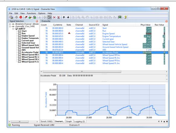
Figure 5.48: Signal module Overwrite View
