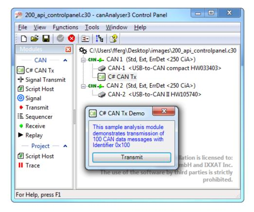
Figure 5.64: Control Panel with "C# CAN Tx" sample analysis module
